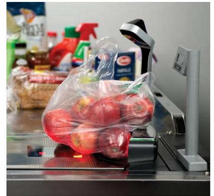
Both scanners are equipped with Datalogic's patented "Green Spot" technology. When a bar code is read, a green spot is projected on the code informing the user of a good read, an advantageous feature for busy supermarkets operating multiple checkout lanes in close proximity to one another.
